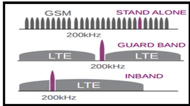
Figure 2: NB-IoT Deployment option [8]
