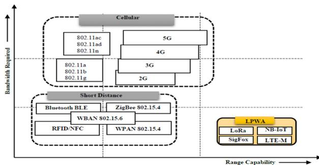
Figure 1: Bandwidth and Range capability for cellular and short distance [6]
