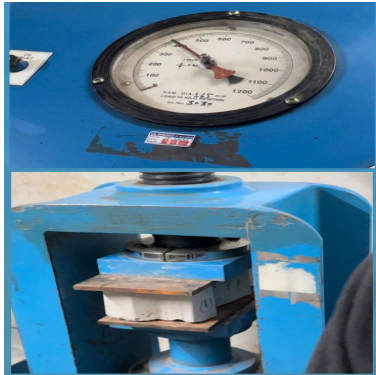
Fig 3: Compressive Test of Paver Block (ZigZag)
