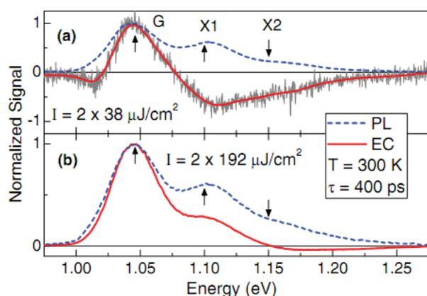
**Figure 4:** Time-integrated PL spectra were recorded at 400 ps and calculated corresponding EC signal for two different excitation pump fluence on the InAs/GaAs QDs sample.<sup>[30]</sup>
