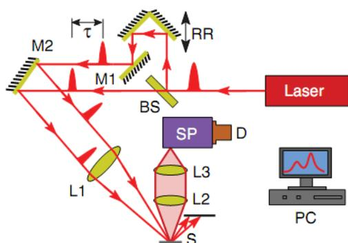
**Figure 3:** Schematic diagram of excitation correlation spectroscopy experimental setup. Symbols: BS:-Beam Splitter, M1-M2: - Mirrors, RR:- Retro Reflector, L-L3: Lenses, SP:- Spectrometer, S:- Sample.<sup>[30]</sup>
