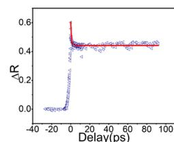
**Figure 2:** The typical time evaluation of differential pump-probe reflectivity signal for heavy-hole exciton observed on 17.5 nm GaAs MQWs sample. Red line represents the double exponential fit to extract the coherence phenomena and life time of heavy-hole-exciton.<sup>[34]</sup>
