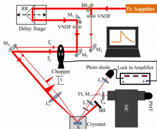
**Figure 1:** Schematic diagram of the Pump-probe differential reflectivity setup. Symbols: BS:-Beam Splitter, M1-M4: -Mirrors, FL M5 :-Flip Mirror, VNDf:- Variable Neutral Density Filter, RR:- Retro Reflector,  $f_1$  and  $f_2$ : chopping frequency, L1-L4: Lenses, BB:- Beam Blocker, MC:-Monochromator, S:- Sample.<sup>[31]</sup>
