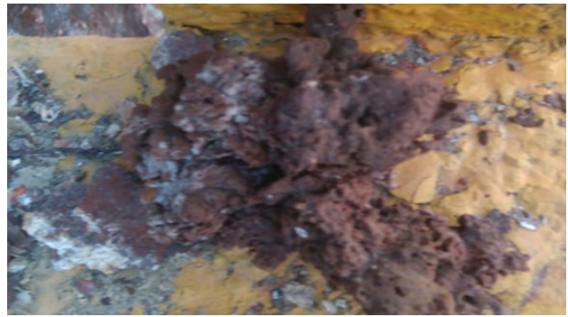
Figure 5: Deposit collected from weep hole
