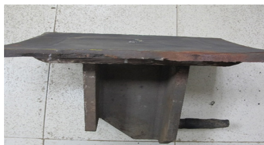
Figure 13: Failure location - fracture surface pad plate side
