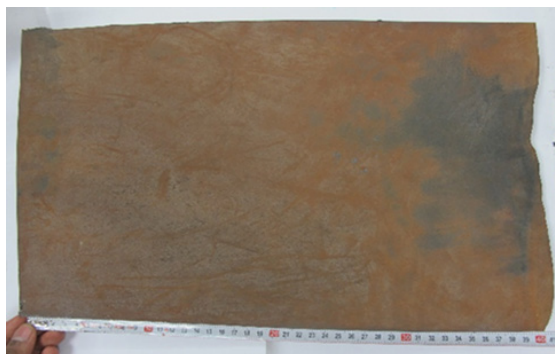
Figure 11: Brownish discoloration on inside surface
