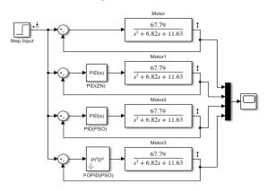
Figure 5: Comparative Simulink model of electric motor.
