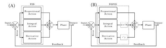
Figure 1: Parallel structure of PID controller, (A) Integer order, (B) Fractional order.
