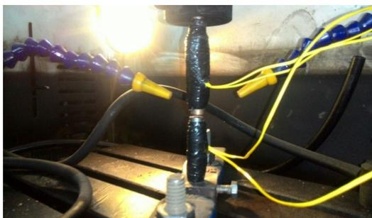
Figure 2: EDM Tool & Work Piece
