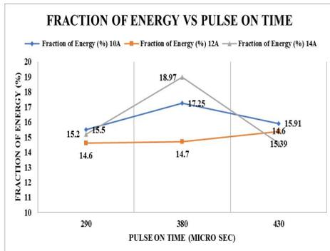
**Figure 8:** Fraction of energy versus Pulse on time at 40 V
