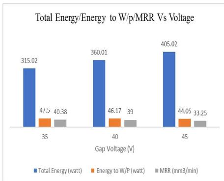
Figure 5: Total Energy/Energy to W/P /MRR Vs gap voltage at 10A & 290µs
