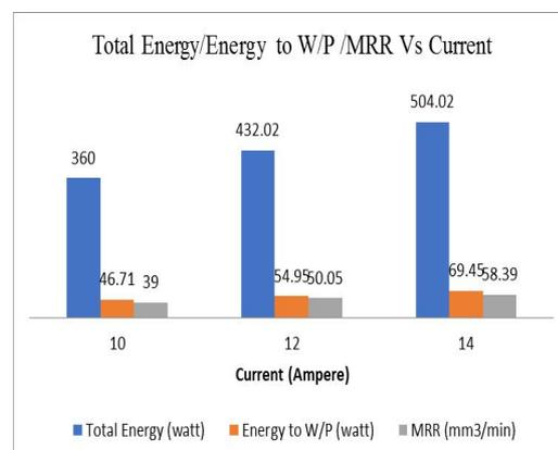
Figure 4: Total Energy/Energy to W/P /MRR Vs Current at 380µs & 40V
