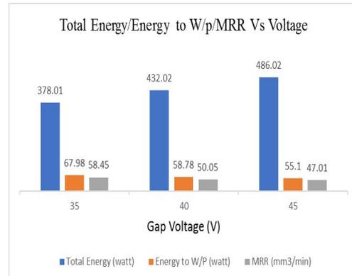
Figure 6: Total Energy/Energy to W/P /MRR Vs gap voltage at 12A & 380µs
