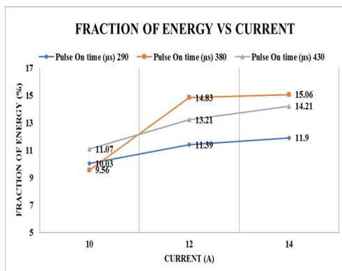
**Figure 9:** Fraction of energy versus Current at 45 V
