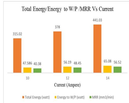
Figure 3: Total Energy/Energy to W/P /MRR Vs Current
