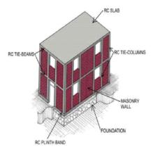
Figure 2: Typical CM building showing its structural elements (Brzev,2007)[5].
