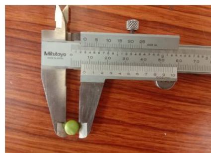
Figure 1: Actual measurement of green pea seeds using vernier caliper
