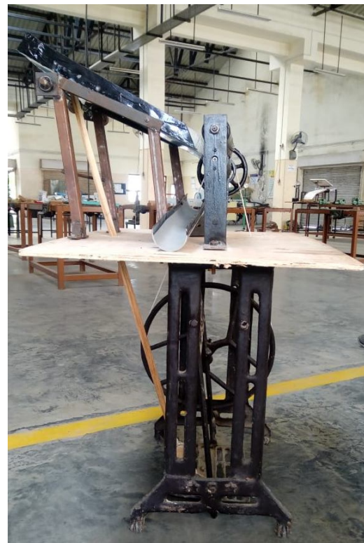
Figure 11: Side View of Developed Green Pea Depoding Machine
