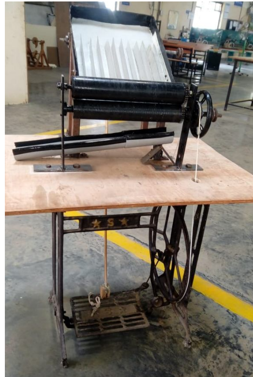
Figure 10: Front view of Developed Green Pea Depoding Machine
