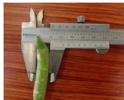
Figure 2: Actual measurement of green pea pods using vernier caliper
