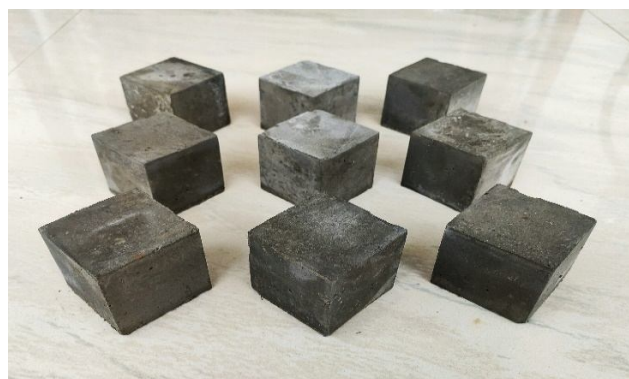
Figure 3: Demoulded Cube Specimens
