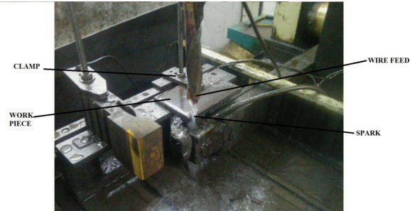
Figure 1: Matching of Die Steel D3 on Electronica Maxicut Wire EDM
