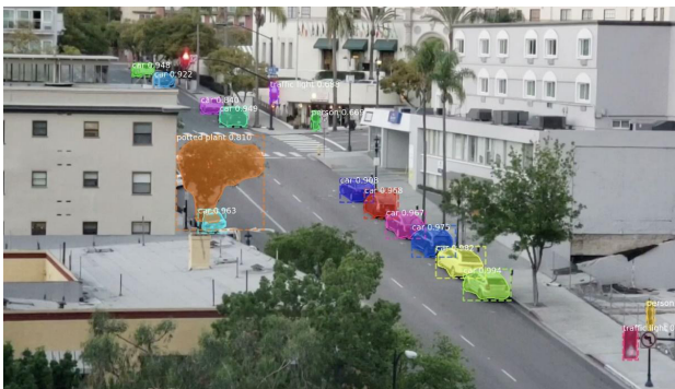
Fig. 3: Image with default COCO objects identified – cars, people, traffic lights and a tree
