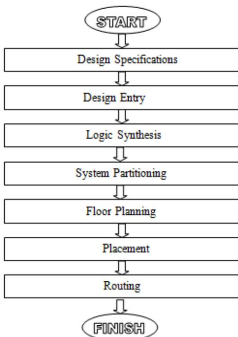
Figure 1: Common ASIC Design Flow
