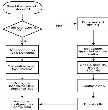
**Figure 6: Configurations for handover**
