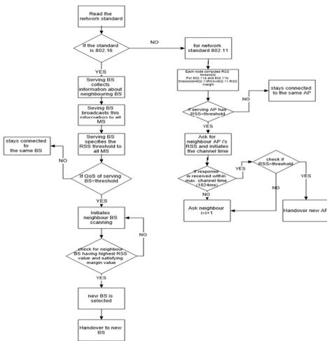
**Figure 5: Phases used to perform handover**
