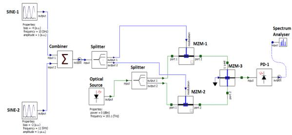
Figure 3 : DPSDMZM modulator simulation using Lumerical interconnect tool
