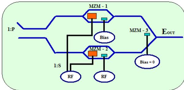
Figure 5: DPSDMZM modulator structure
