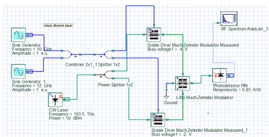
**Figure 1** : DPSDMZM using Opti-system for linearization
