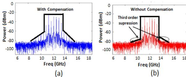
Figure 6 : Multi tone signals with and without non-linearity compensation
