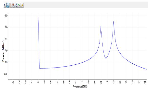
Figure 4 : MZM modulator output after IMD3 compensation
