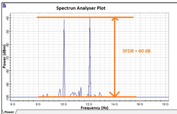
Figure 2 : Linearized RF output signal at the modulator output
