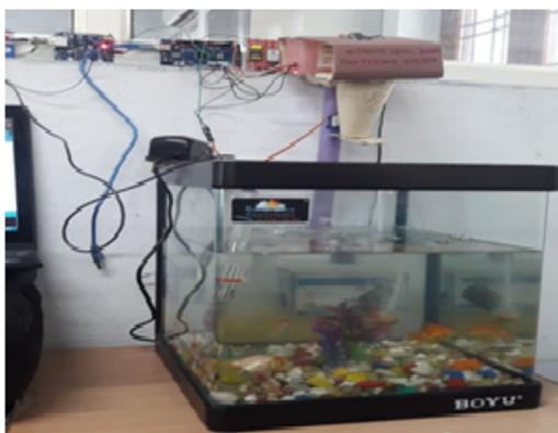
Figure 5: Prototype of Fish feeding system
