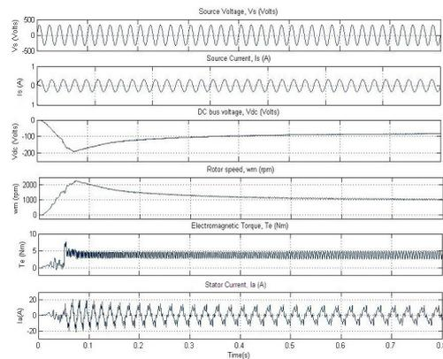
**Figure 4:** Dynamic Characteristics of the drive during start-up from  $V_{dc} = 0V$  to 75V
