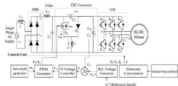
**Figure 1:** A CSC converter-fed Sensor-less brushless DC Motor Drive System
