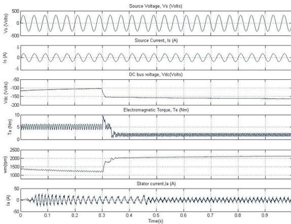
Figure 5: Dynamic Characteristics of the drive during step-change in  $V_{dc}$  from 100V to 150V
