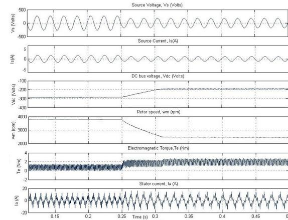
Figure 6: Dynamic Characteristics of the drive during a step-change in  $V_s$  from 270V to 180V
