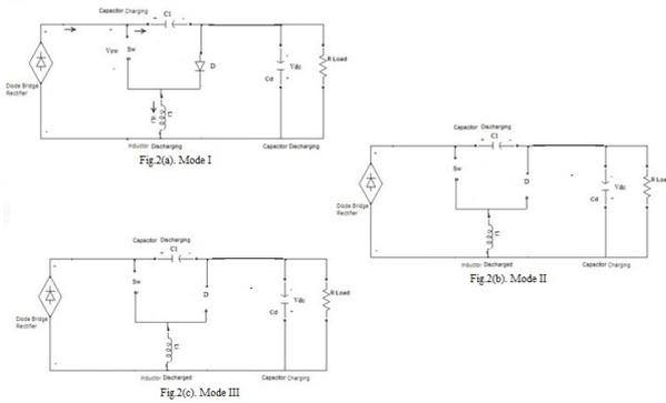
**Figure 2:** Operational Modes of a CSC converter
