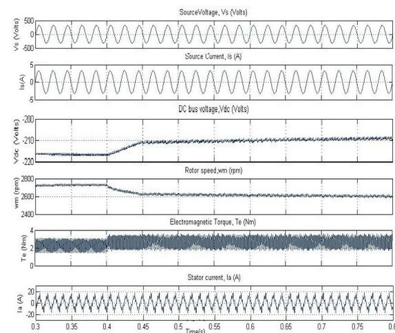
Figure 7: Dynamic Characteristics of the drive during step-rise in load torque from 0.4Nm to 0.8Nm
