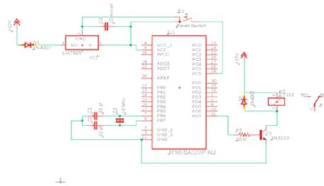
Figure 8: Ignition Control Circuit
