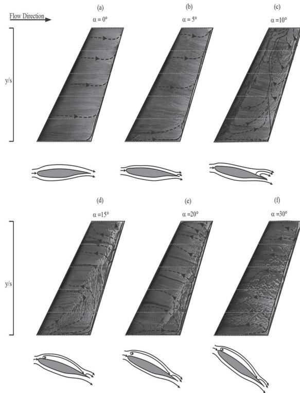
**Figure 4:** Surface Flow Visualization Pattern With Schematic Sketches Over Leeward Surface of Swept-Back, Tapered Wing Model
