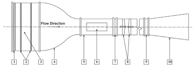
[1] Honeycomb, [2] Screens, [3] Settling chamber, [4] Contraction Cone (9:1), [5] Test Section (SQ 600X600mm), [6] Transparent Panel, [7] Transition Piece, [8] Fan, [9] Damper, [10] Diffuser
