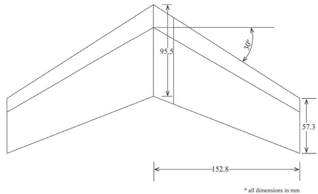
Figure 3: Geometry of Wing Model
