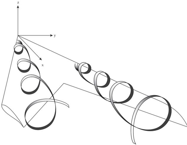
Figure 1: Schematic of swept-back, tapered wing vortex flow
