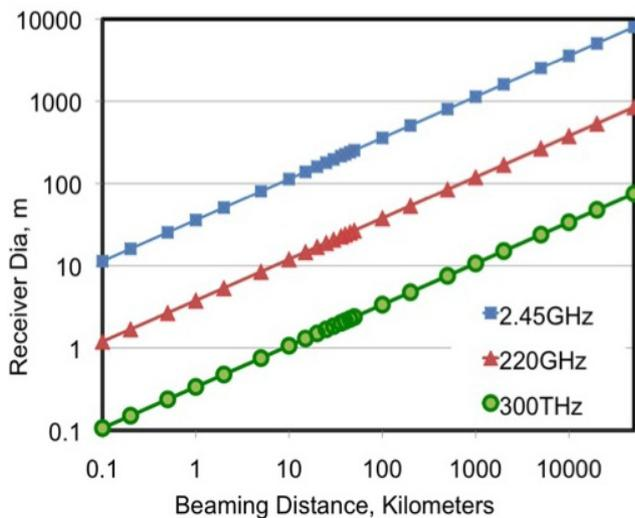
**Fig.2.** Receiver Dia Vs Beaming Distance, for Different Frequencies
