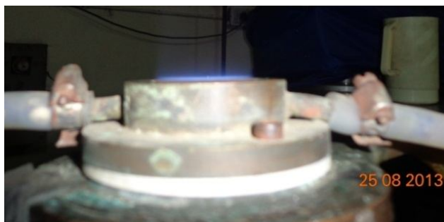
Fig. 2. Direct photograph of stoichiometric Hythane (10% H 2 -90% CH 4 )-Air mixture at p=1 bar and T=292 K
