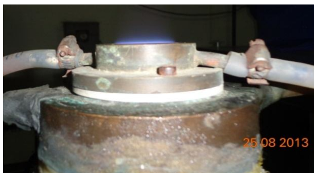
Fig.4. Direct photograph of stoichiometric Hythane (30% H 2 -70% CH 4 )-Air mixture at p=1 bar and T=292 K
