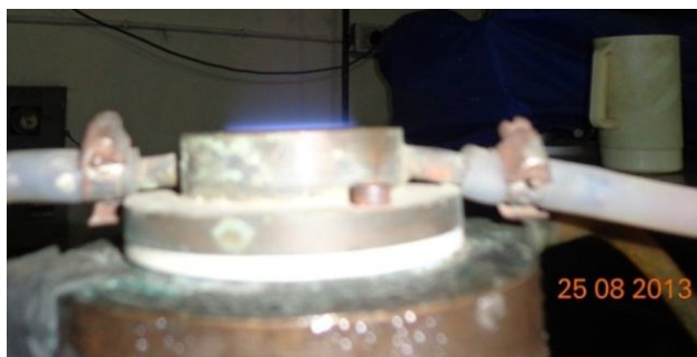
Fig.3. Direct photograph of stoichiometric Hythane (20% H 2 -80% CH 4 )-Air mixture at p=1 bar and T=292 K
