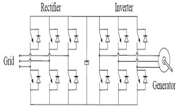
Fig. 11. The back-to-back PWM-VSI converter topology
