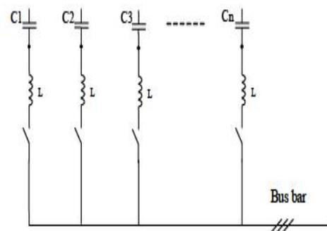
Fig.9. Capacitor bank configuration for power factor compensation in a wind turbine
