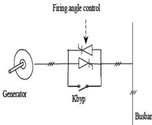
Fig. 7. Connection diagram of soft starter with generators.
