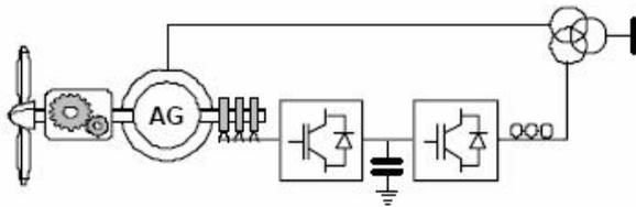
Fig.4. Doubly Fed Wound Rotor Induction Generator
