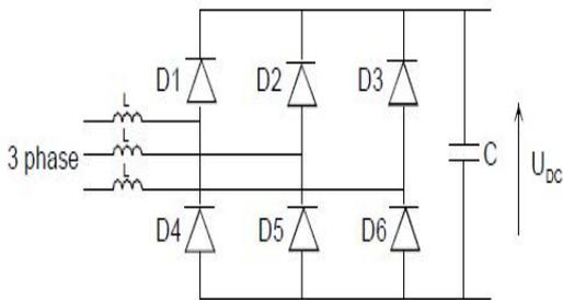
Fig. 10. Diode rectifier for three-phase ac/dc conversion
