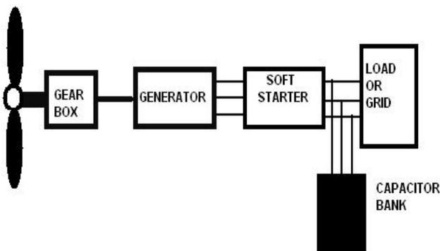
Fig .5. General arrangement of fixed-speed generation system
