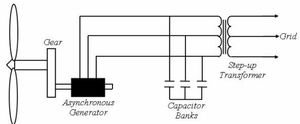
Fig .5. Variable Speed Squirrel Cage Induction Generator
