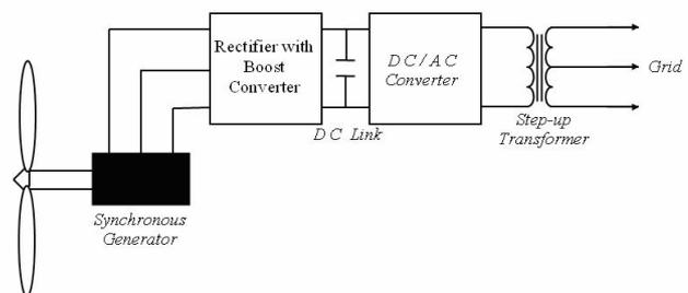
Fig. 2. Permanent-Magnet Synchronous Generator with a Boost Chopper
