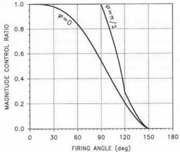
Fig. 8. Control characteristic for a fully controlled soft starter
