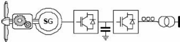
**Fig.3.** Permanent-Magnet Synchronous Generator with PWM converter
