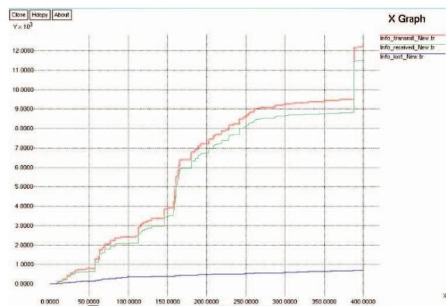
Fig. 2. Shows transmit, received lost packet and drop packet in route advertisement.
