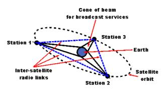
Fig.7. Arthur C Clarke's Geostationary Orbiting Satellites Concept
