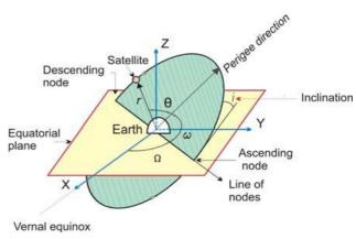
Fig. 6. Space Orbital Parameters
