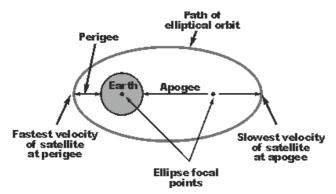
Fig. 4. Highly Elliptical Satellite Orbit, HEO
