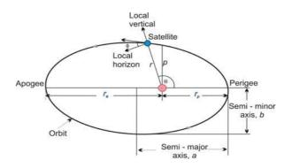
Fig. 5. Major Parameters of an Elliptical Orbit
