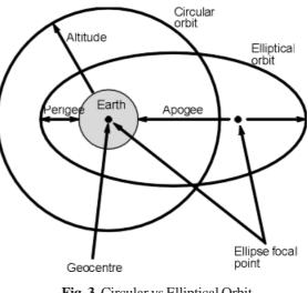
Fig. 3. Circular vs Elliptical Orbit
