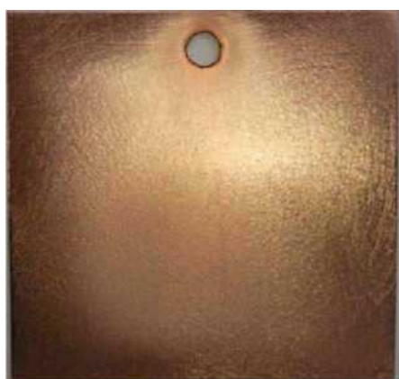
Fig.3: Appearance of correct bright copper coated in with bright coat using PV panels
