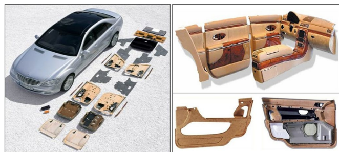
Figure 1 : Automotive components manufactured from polymer composites reinforced with plant-based natural fibres. [44]
