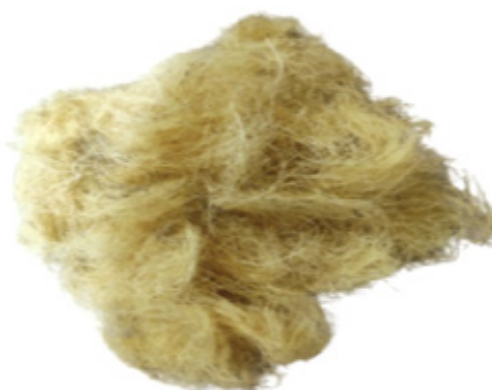
Figure 3: Chemically treated coir fibre
