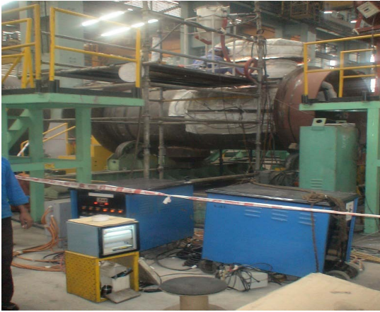
Figure 5: Preheating arrangement- Nozzle welds
