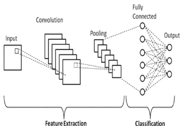
Figure 3: Block Diagram Of CNN
