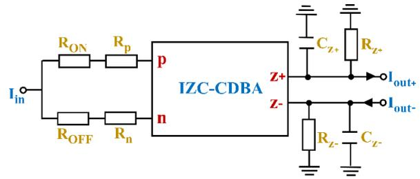
Figure 6: Equivalent circuit reveals parasitics during positive cycle
