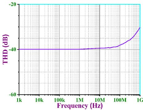
**Figure 15:** Variation of THD of the proposed full-wave rectifier as a function of frequency with CMOS based IZC-CDBA
