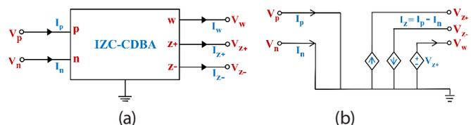
**Figure 1:** The IZC-CDBA building block (a) Block diagram (b) Equivalent circuit
