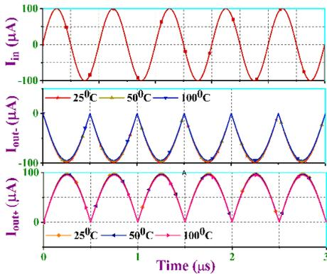
**Figure 11:** Simulated responses at different temperatures for the designed full-wave rectifier with CMOS based IZC-CDBA
