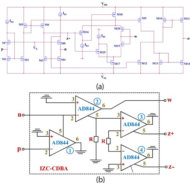
Figure 2: Internal structure of IZC-CDBA building block (a) CMOS based structure (b) IC AD844 based structure
