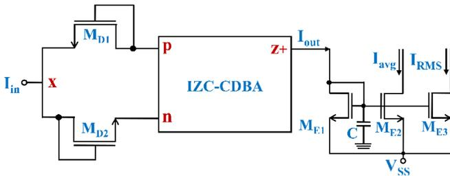
Figure 22: The proposed full-wave rectifier based average and RMS value computation circuit for sinusoidal wave
