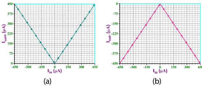
**Figure 7:** DC transfer characteristics of the suggested full-wave rectifier circuit with CMOS based IZC-CDBA (a) Non-inverting output (b) Inverting output
