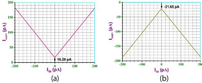
**Figure 19:** DC transfer characteristics near zero crossing region of the suggested rectifier with AD844 based IZC-CDBA (a) Non-inverting output (b) Inverting output
