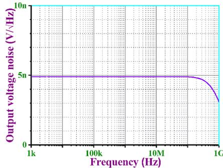
**Figure 16:** Variation of output noise of the proposed full-wave rectifier against frequency with CMOS based IZC-CDBA
