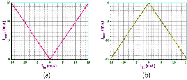
**Figure 18:** DC transfer characteristics of the suggested full-wave rectifier circuit with AD844 based IZC-CDBA (a) Non-inverting output (b) Inverting output
