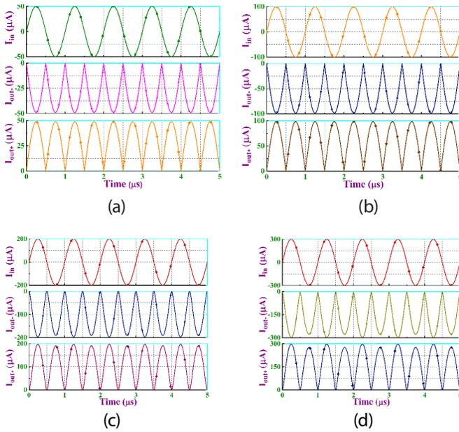
**Figure 10:** Simulated rectified outputs of the suggested full-wave rectifier circuit with CMOS based IZC-CDBA for different input current amplitudes in dual phase at 1 MHz frequency (a) 50  $\mu\text{A}$  (b) 100  $\mu\text{A}$  (c) 200  $\mu\text{A}$  (d) 300  $\mu\text{A}$
