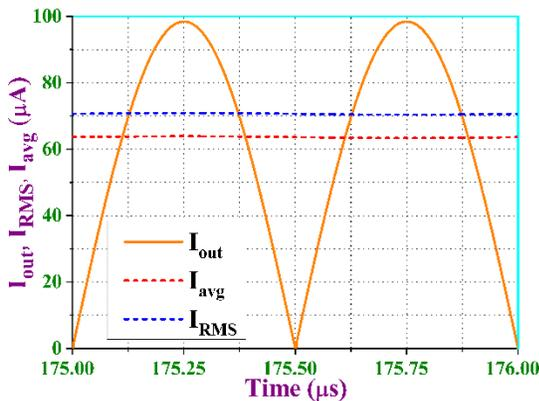
Figure 23: Simulated  $I_{\text{out}}$  (rectified),  $I_{\text{RMS}}$  and  $I_{\text{avg}}$  for a 100  $\mu\text{A}$ , 1 MHz sinusoidal input with CMOS based IZC-CDBA
