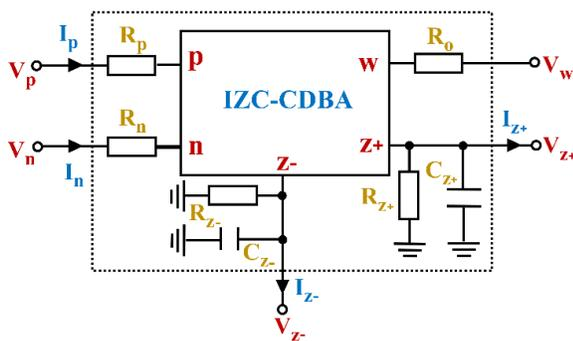
Figure 5: Parasitic model of IZC-CDBA
