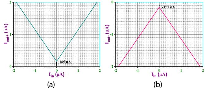
**Figure 8:** DC transfer characteristics near zero crossing region of the suggested rectifier circuit with CMOS based IZC-CDBA (a) Non-inverting output (b) Inverting output
