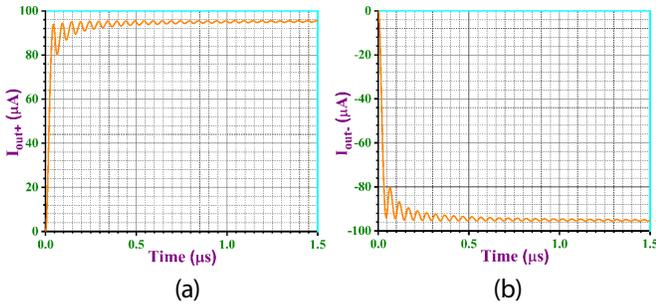
**Figure 14:** Average DC current output of the proposed full-wave rectifier with CMOS based IZC-CDBA for dual phase (a) Non-inverting output (b) Inverting output
