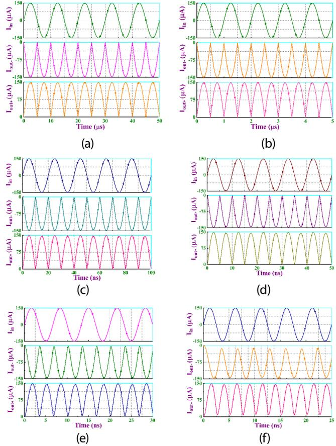
**Figure 9:** Simulated rectified outputs of the suggested rectifier with CMOS based IZC-CDBA at different frequencies in dual phase for input current of 150  $\mu\text{A}$  peak value (a) 100 kHz (b) 1 MHz (c) 50 MHz (d) 100 MHz (e) 150 MHz (f) 200 MHz
