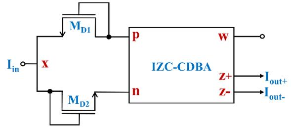
Figure 3: The proposed current-mode precision full-wave rectifier
