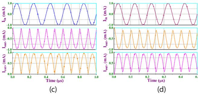
**Figure 20:** Simulated rectified outputs of the suggested full-wave rectifier circuit with CMOS based IZC-CDBA at different frequencies in dual phase for input current of 1 mA peak value (a) 100 kHz (b) 1 MHz (c) 5 MHz (d) 10 MHz
