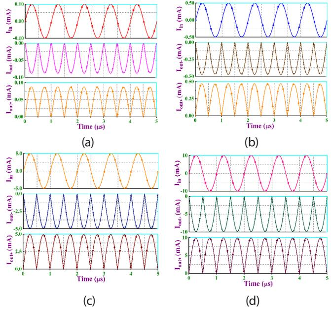
**Figure 21:** Simulated rectified outputs of the suggested full-wave rectifier circuit with AD844 based IZC-CDBA for different input current amplitudes in dual phase at 1 MHz frequency (a) 0.1 mA (b) 0.5 mA (c) 5 mA (d) 10 mA
