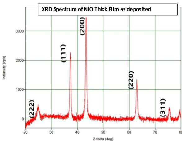
**Figure 1:** XRD pattern at firing temperatures(400°C)
