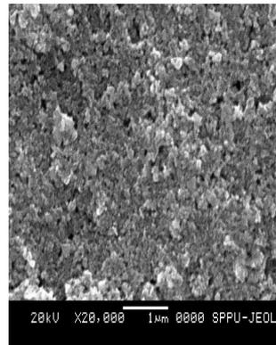
**Figure 2a:** SEM images of NiO thick films when film is unannealed
