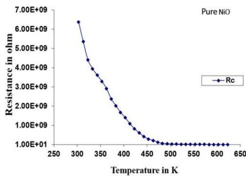
**Fig. 4(a):** Plot of resistance against temperature for pure NiO thick films at 400°C
