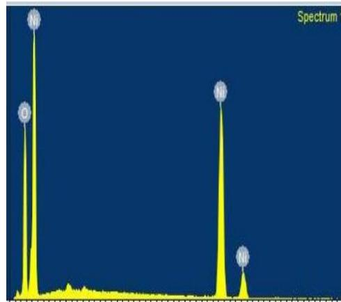
**Figure 3:** EDAX of NiO Thick film at 400 °C
