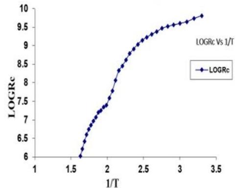
**Fig. 4(b):** Plot of logR against 1/T NiO thick films annealed at 400°C for activation energy
