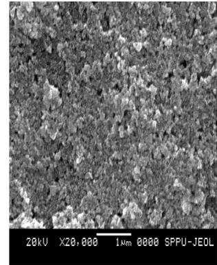
**Figure 2b:** SEM images of NiO thick films: film is annealed at 400°C
