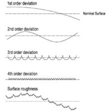
Figure 2: Surface Roughness form Deviations [11]
