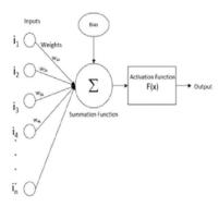
Figure 2: Structure of a singular neuron used in ANN [36]
