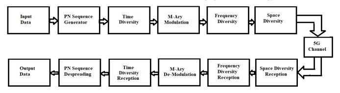
Figure 1: Basic architecture of 5G system
