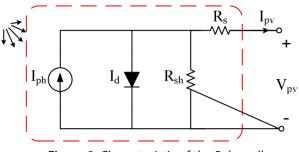
Figure 2: Characteristic of the Solar cell
