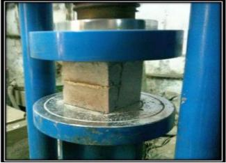
Figure 1: Compression Testing Equipment
