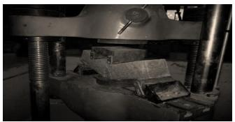
Figure 2: Flexural test equipment
