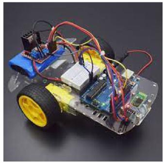
Figure 4: Android controlled robot car
