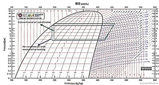
**Figure 6:** P-h chart of the conventional and retrofitted system with pad thickness 1 inch at Tamb. 30°C.
