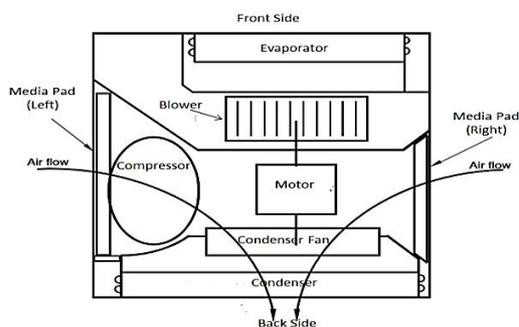
Figure 4: Aerial image of an air conditioner equipped with an evaporative cooling system [5]
