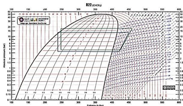
**Figure 7:** P-h chart of the conventional and retrofitted system with pad thickness 2 inches at Tamb. 30°C
