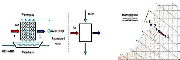
**Figure 1:** Working principle of DEC and its representation on the psychrometric chart [1]
