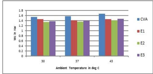
**Figure 9(a):** Comparison of compressor work with and without evaporative cooling
