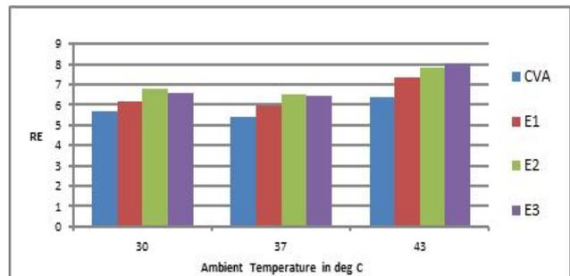
**Figure 9(b):** Comparison of refrigerating effect with and without evaporative cooling.
