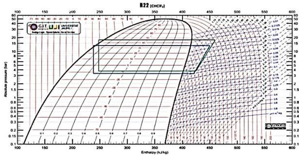
**Figure 8:** P-h chart of the conventional and retrofitted system with pad thickness 3 inches at Tamb. 30°C
