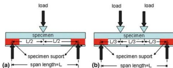
Figure 5: Arrangement for bend test [2]
