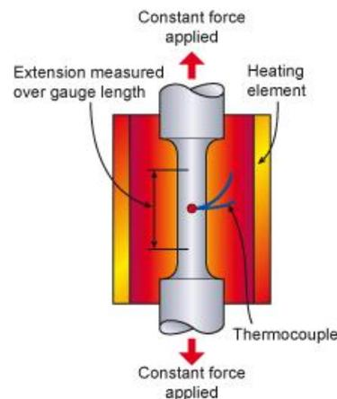
Figure 2: Specimen for creep test [7]
