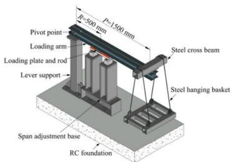
Figure 4: Flexural test apparatus [10]
