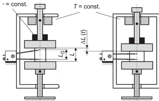
Figure 3: Creep Testing Machine [10]
