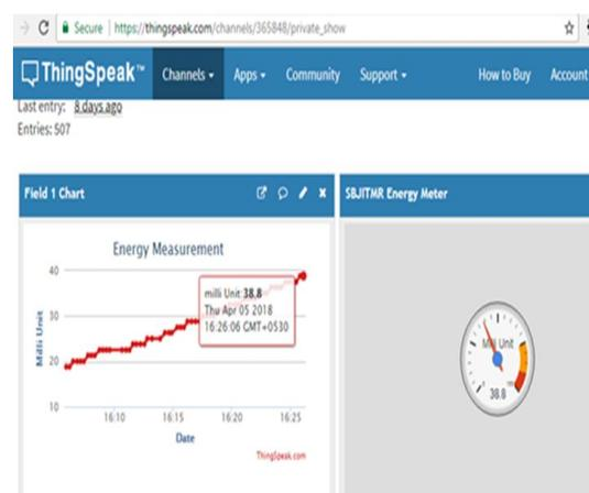
Figure 6: Energy consumption reading at different instant on ThingSpeak website
