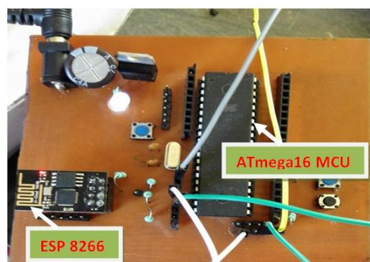
Figure 4: Developed IoT Board
