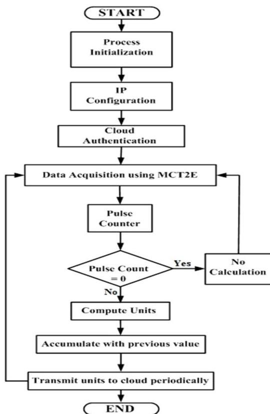
Figure 3: System work flow chart
