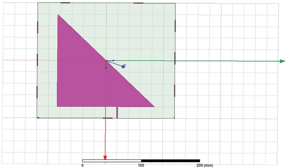
**Figure 1:** Triangle shaped antenna
