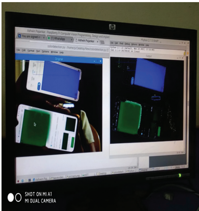
Figure 7: Both Green and Blue Colors Are Detected
