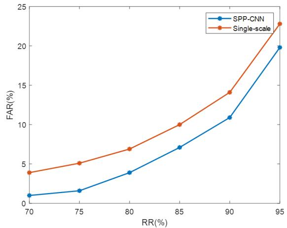
Figure 3: FAR and RR for detecting vehicle using image of single scale
