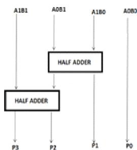
**Figure 1:** 2-Bit x 2-Bit Vedic Multiplier
