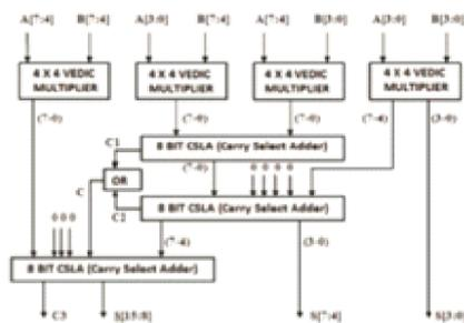
Figure 3: 8-Bit X 8-Bit Vedic Multiplier
