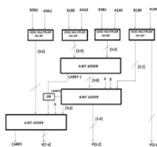
**Figure 2:** 4-Bit x 4-Bit Vedic Multiplier
