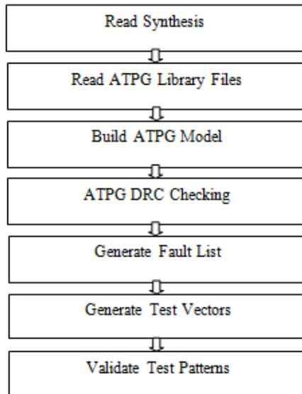
Figure 4: Flow Chart of ATPG simulation phase
