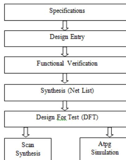
Figure 2: DFT Design flow in ASIC
