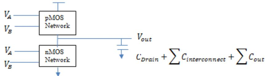
**Figure 5:** Representation of switching power calculation in CMOS logic gate.
