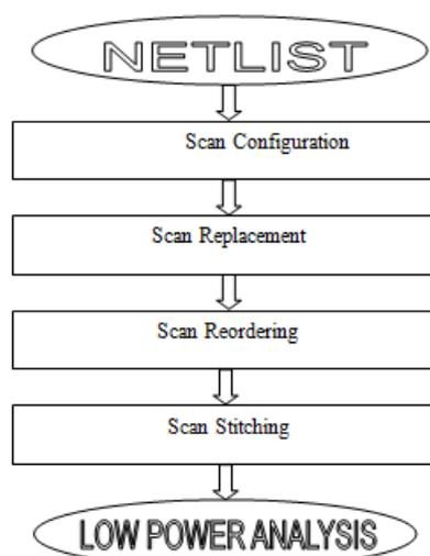
Figure 3: Flow chart of Scan Synthesis Phase
