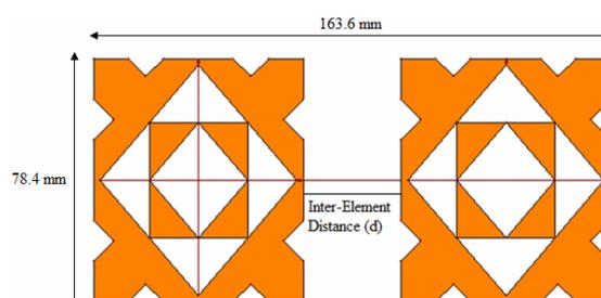
Figure 3: Spatial Arrangement of Fractal Antenna Elements for MIMO System
