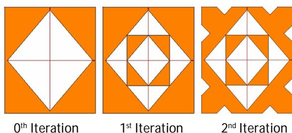
Figure 1: Three Iterations of Hybrid Fractal Boundary Antenna Element
