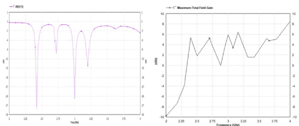
**Figure 4:** Return Loss Curve and Total Field Gain Curve for Second Iteration Geometry
