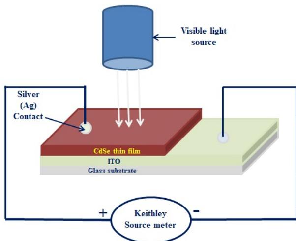
**Figure 3:** Schematic diagram of Ag/CdSe/ITO Schottky device structure.
