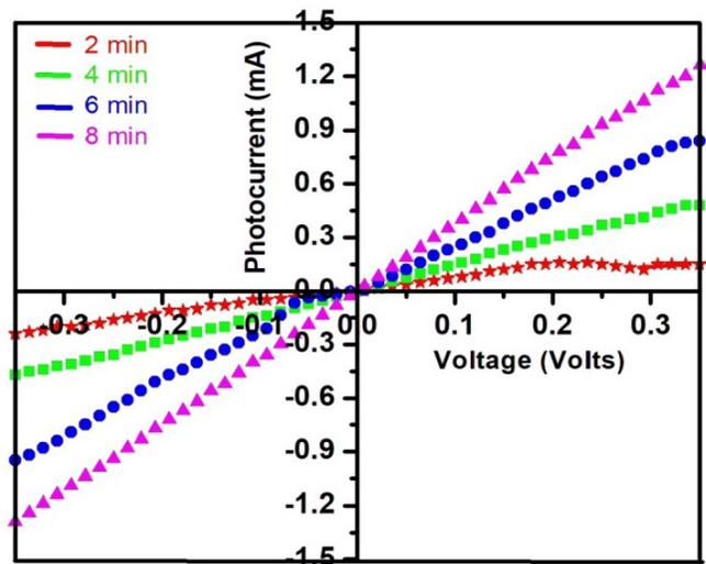
Figure 7: Plot of photocurrent versus voltage for Ag/CdSe/Ag M-S-M structure.
