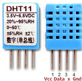
Figure 5: DHT11 humidity sensor
