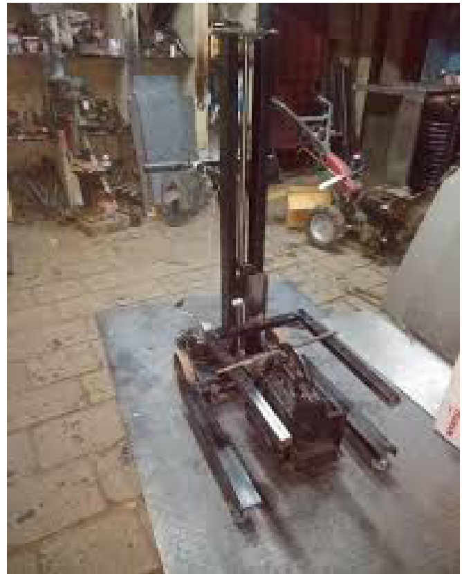
Figure 3: Forklift using lead screw mechanism
