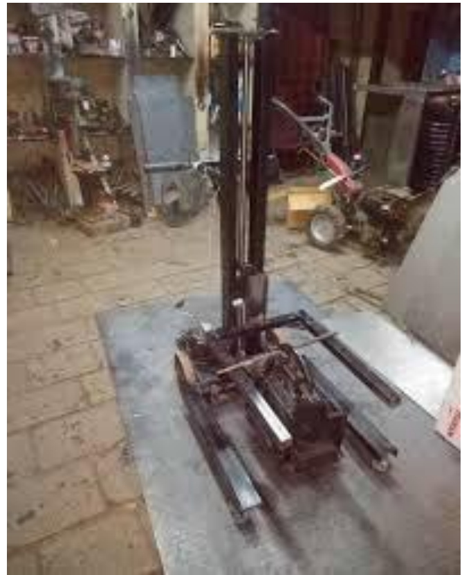
Figure 3: Forklift using lead screw mechanism
