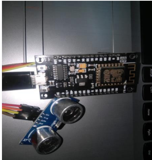
Figure3.2 : Connection of ultrasonic sensor with node ncu
