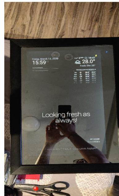
Figure 4.1: Two-way mirror with display on.
