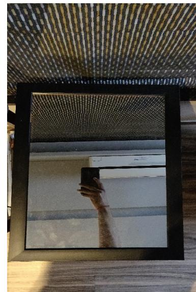
Figure 4.2: Two-way mirror with display off.
