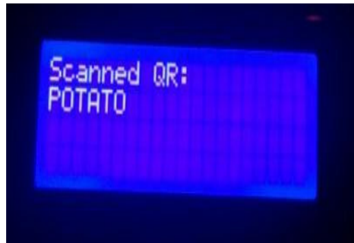
Figure 3 and 4: The system scans the QR code of the item using the camera module and detects the item.
